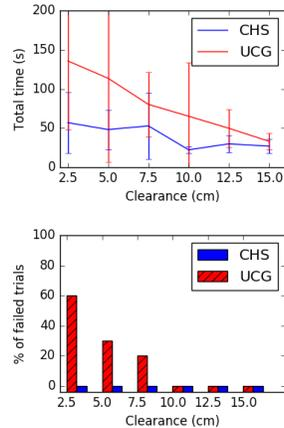
Fig. 6: Total time and failure % for R4, averaged over 10 trials for each clearance with a 5 min. timeout
