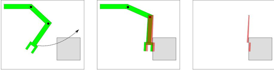
Fig. 1: A plan for the green robot (left) results in a collision with the grey unknown obstacle. A red collision hypothesis set is added using links possibly in collision based on measured joint torques (center). The known free space is removed (right).
