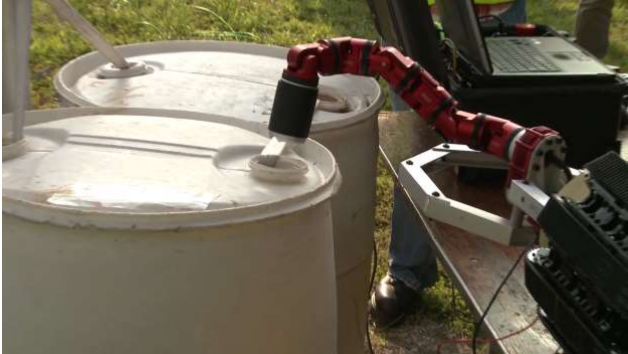
Fig. 5. The series elastic modules are configured into an articulated arm that is readily attached to a mobile base. The end effector, containing a camera and laser range sensor, can be used to inspect confined spaces.
