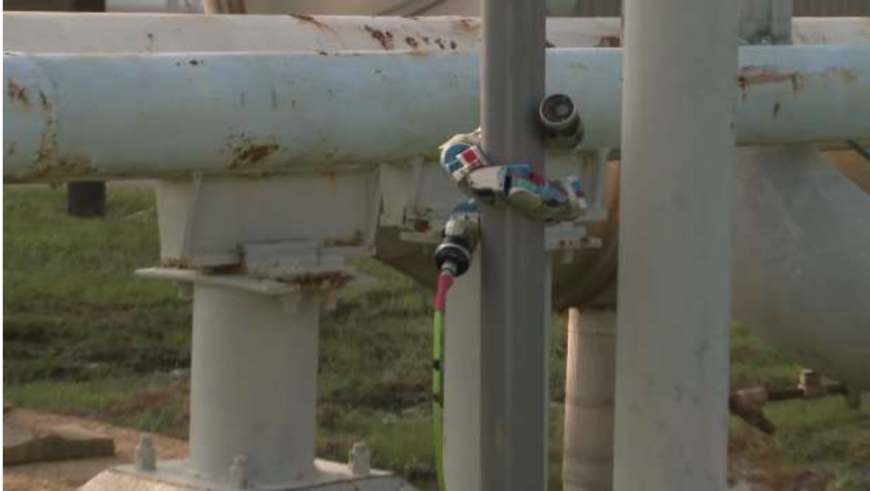
Fig. 2. The snake robot, shown here at the Portsmouth Gaseous Diffusion Plant, can climb on the inside or outside of pipes by rolling in a helix shape. At a desired vantage point, a user can teleoperate the front joints to aim the camera, while the remaining joints hold the pole.
