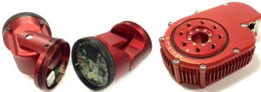
Fig. 1. Our set of modular hardware includes active modules, passive structural elements, and sensors (top) [3]. Our newest platforms are composed of 1 degree-of-freedom actuated S-modules (bottom left [2]) and X-modules (bottom right) from HEBI Robotics ( hebirobotics.com ), a company started by former lab members.
