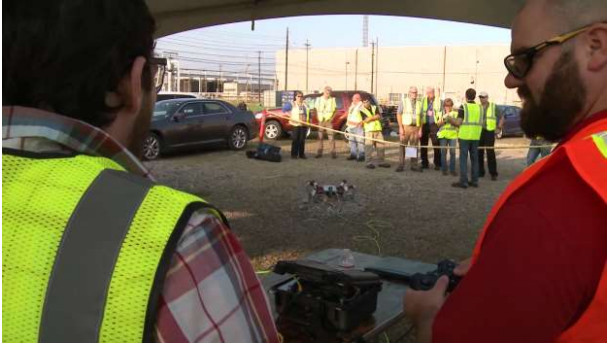
Fig. 4. A U.S. Department of Energy worker drives the hexapod robot at the Portsmouth Gaseous Diffusion Plant using a gamepad controller. The robot is controlled using high-level commands, while low-level controllers use proprioceptive feedback to react to external disturbances and rough terrain.
