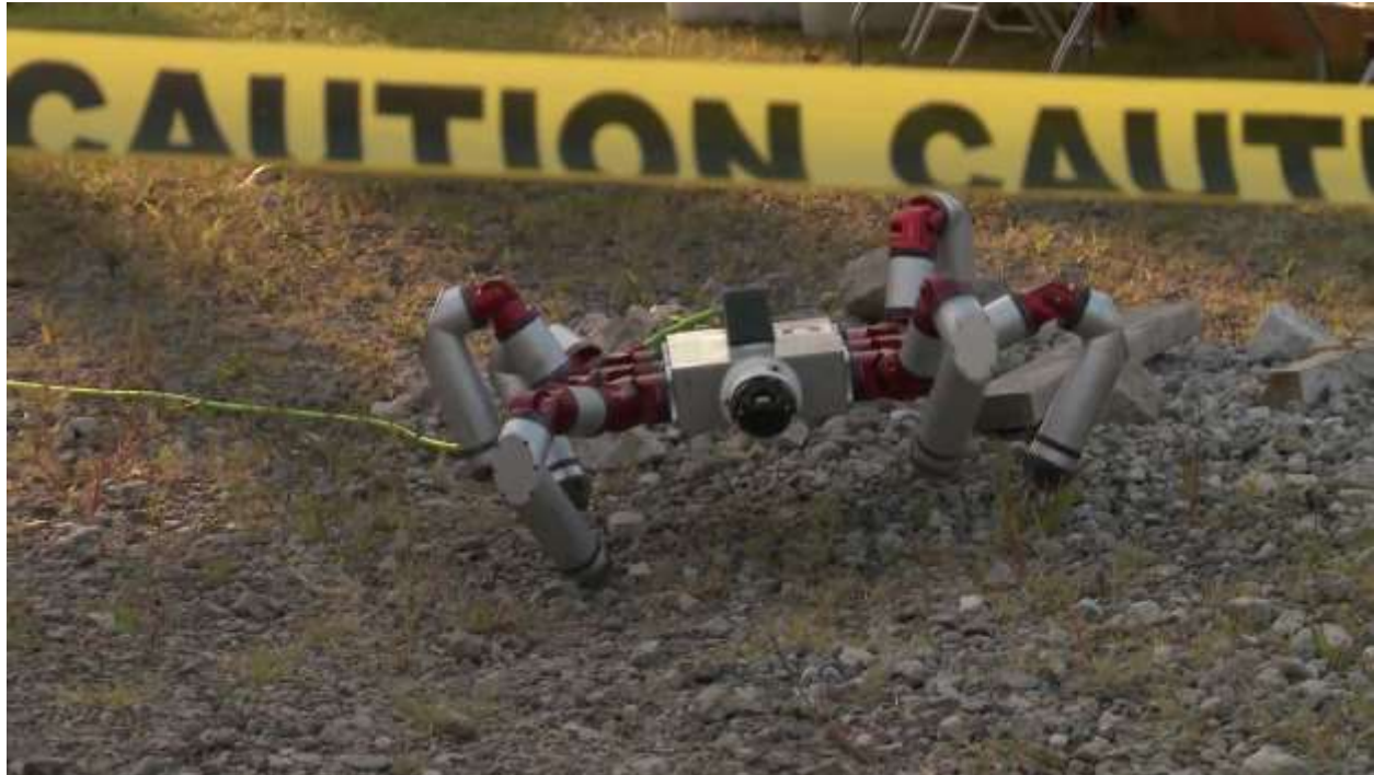
Fig. 3. The hexapod robot walks through piles of rocky debris at the Portsmouth Gaseous Diffusion Plant. A camera is mounted to the head in the configuration depicted; however, its modular design allows any type of end effector, limb, or sensor to be easily attached.
