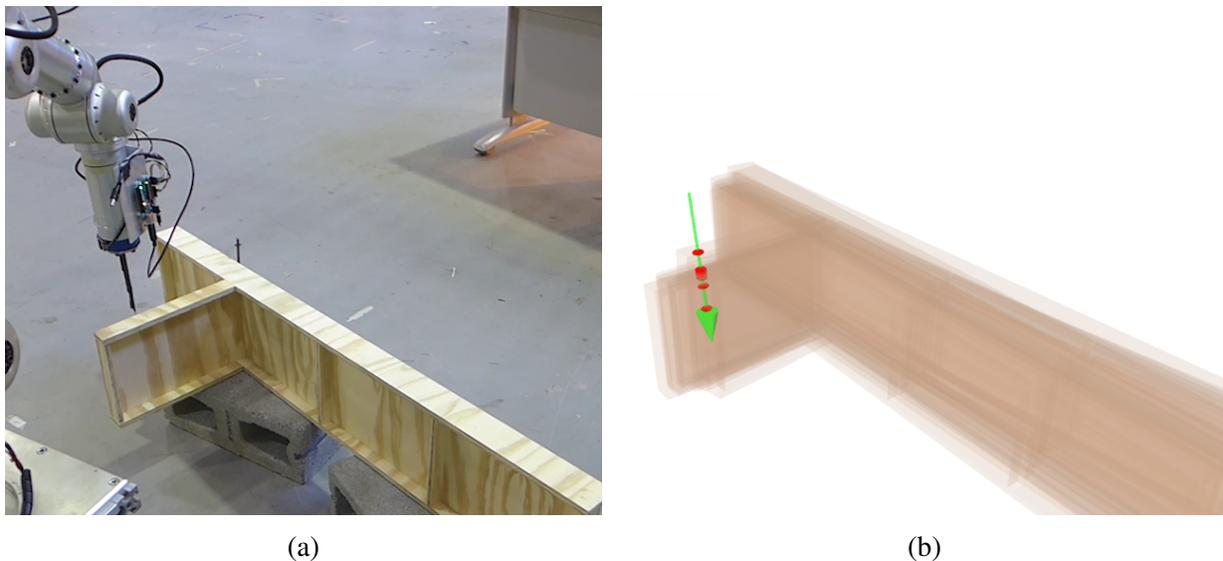
Figure 1.4: **(a)**: The robot performing a touch measurement
