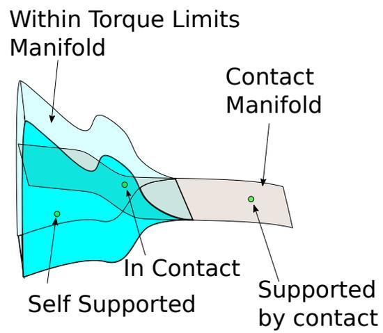
Figure 4.7: Illustration of valid configuration space for an arm potentially supported by contacts
