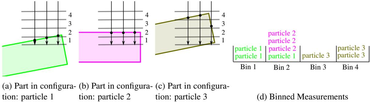
Figure 3.3: Binning of potential measurement on particles for use in calculating information gain. The three arrows represent the nominal measurement action  $\mathcal{M}$  with simulated deviation  $\delta_j$ . The horizontal lines divide the measurement values into the numbered bins.
