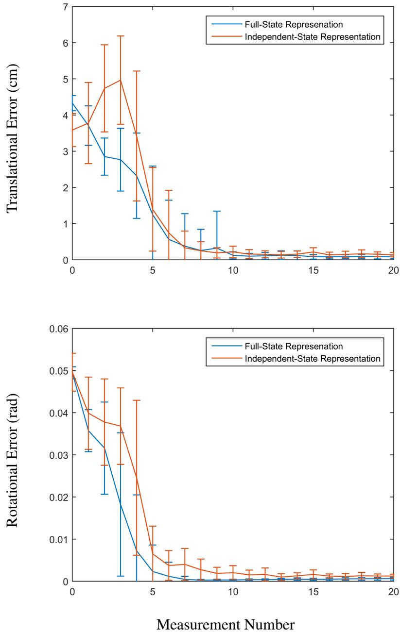
Figure 3.6: Comparison of the accuracy of the update step when using full-state particle filter and independent-state particle filter
