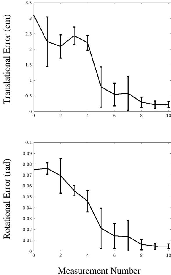
Figure 3.5: Translational and rotational error during localization on the physical robot
