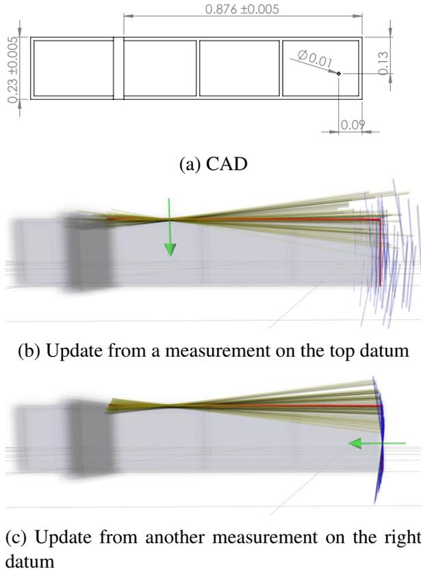
Figure 3.2: Visualization of independent-state particle filter
