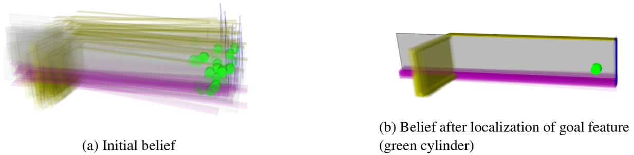
Figure 3.1: Visualization of the belief of the pose of all sections of the part. The green cylinder is the important section to localize and is defined in space through offsets from the top, right, and front faces.
