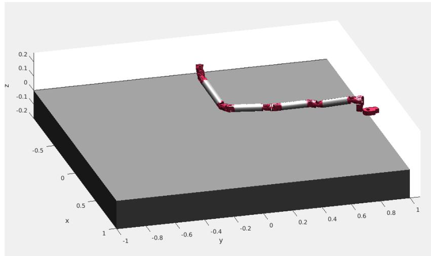
Figure 4.9: Final state of the “optimization with contacts” plan for the snake-like arm reaching far from the base, supported by the environment
