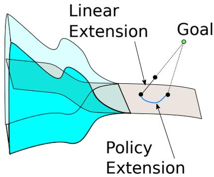
Figure 4.8: Illustration of Policy RRT extension on the contact manifold
