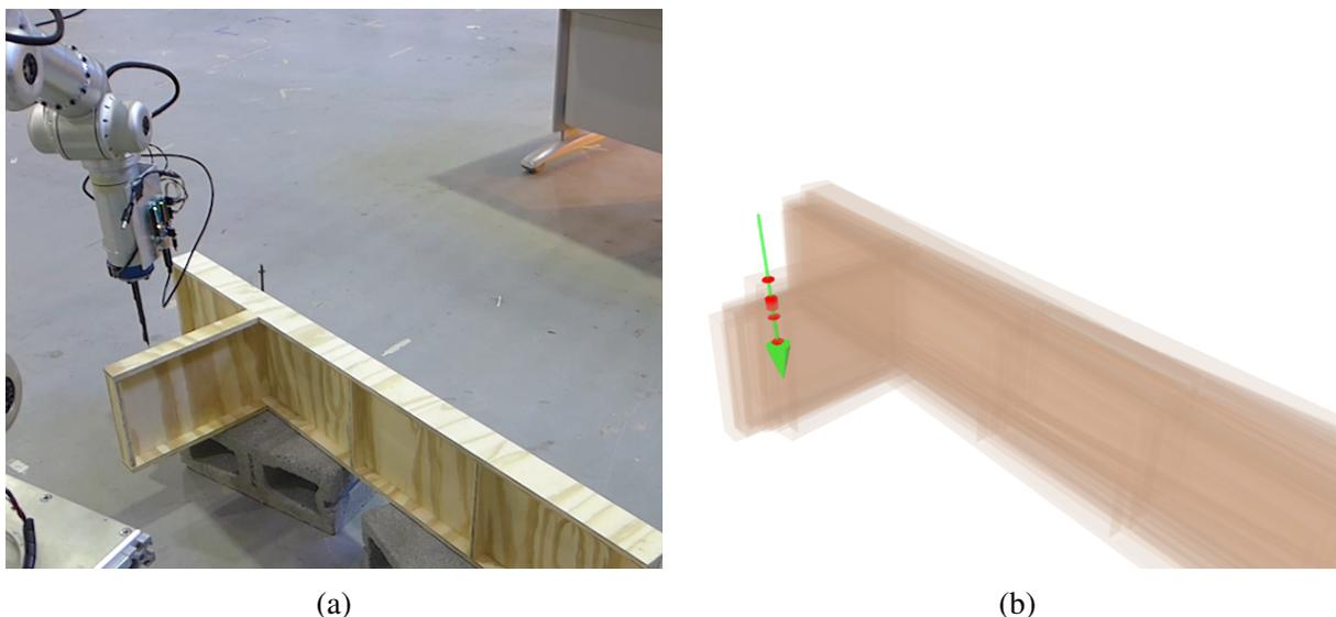
Figure 1.4: **(a)**: The robot performing a touch measurement
