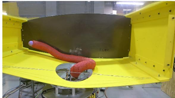
Figure 4.10: Simulated (left) and actual (right) snake arm robots executing motions planned in a model of an airplane wing section
