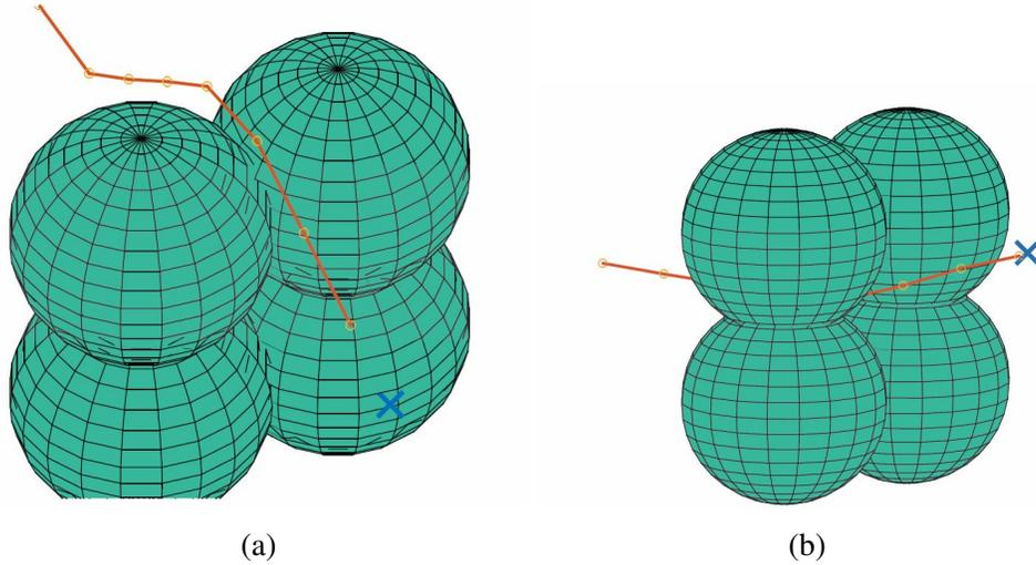
Figure 4.6: The final state of an optimized trajectory finding a local minimum (a) and the global minimum (b) for an arm attempting to reach the blue “X”, through a tight space between 4 spheres
