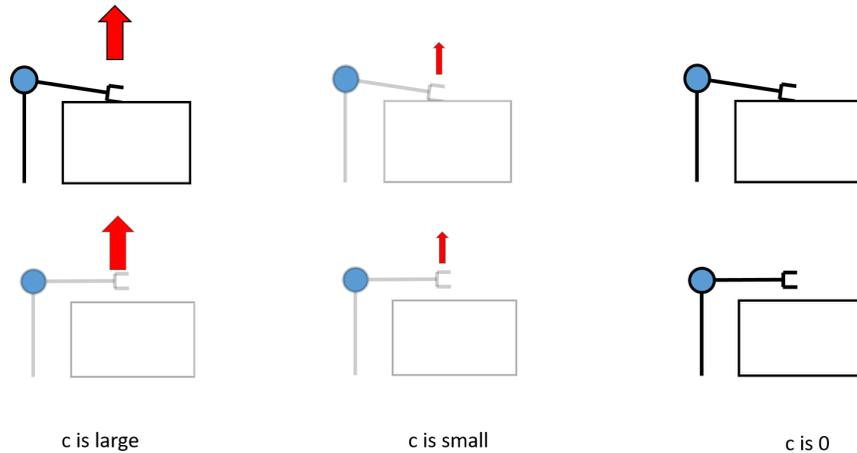
Figure 4.4: Arm configuration and simulated (not realistic) contact forces for a variety of arm configurations and continuous contact variables
