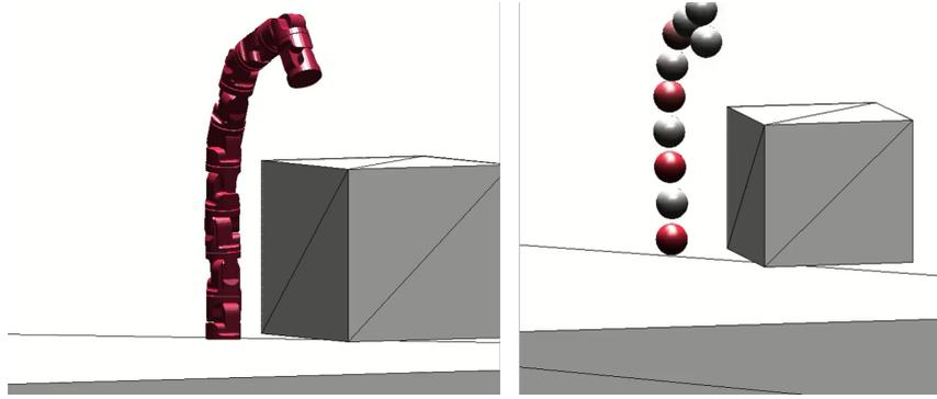
Figure 4.1: The visually accurate robot model (left) and the spherical approximation (right)
